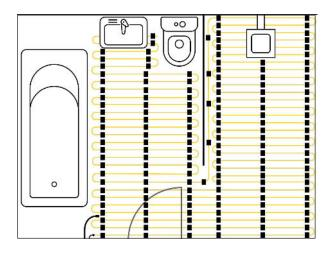
Thermowire loose wire systems are supplied with a roll of cloth tape for taping the cable to the substrate. We mark the ½ way point of the cable to help the installer to ensure he is on track with his spacing of the cable and Thermowire features a 5metre cold tail to ensure an easier install.
