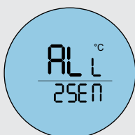
Air Sensor with Floor Limit (All)
